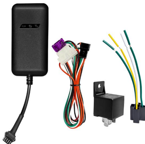
Figure 2 GT02D high precision GPS tracker and accessories
