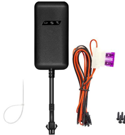
Figure 1 GT02A high precision GPS tracker and accessories
